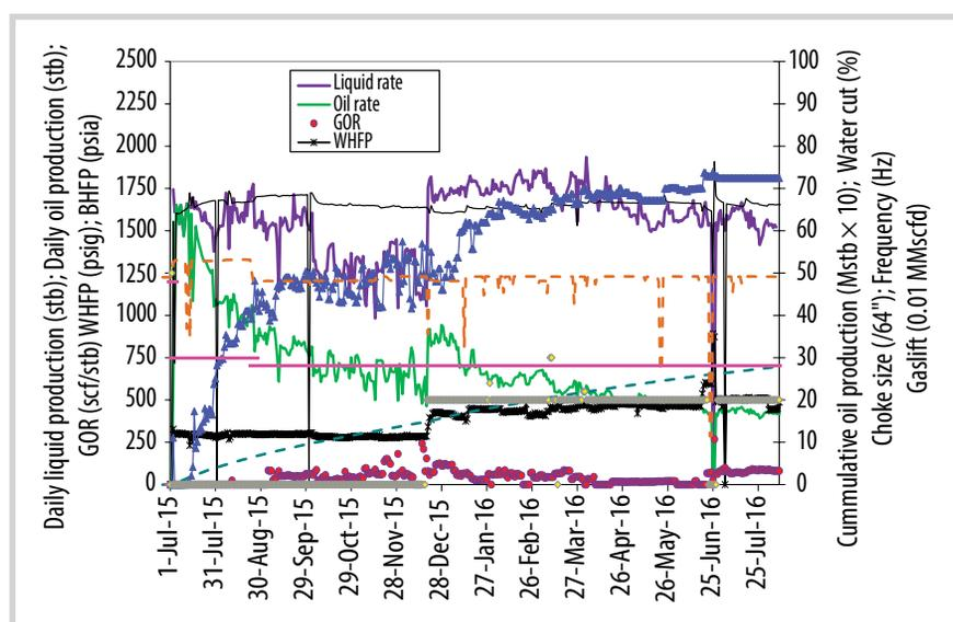
Figure 15. Well production performance with ESP & gas-lift combination.
