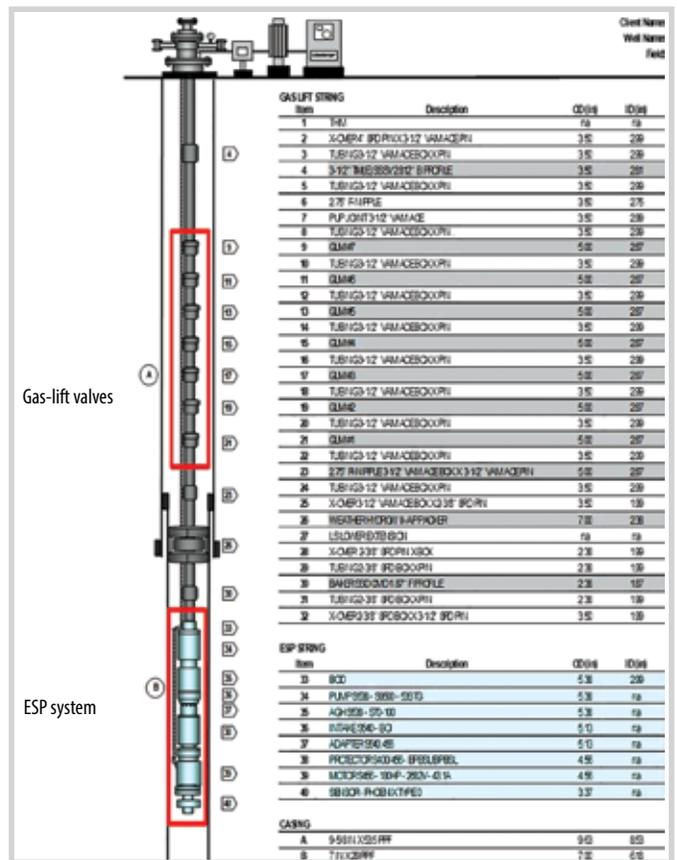
Figure 7. ESP and GL combination system schematic.
